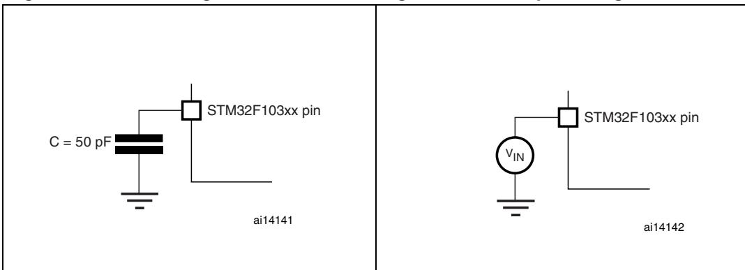
**Figure 11. Pin input voltage**
