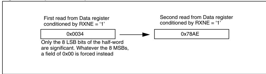
**Figure 234. LSB Justified 16-bit extended to 32-bit packet frame with CPOL = 0**
