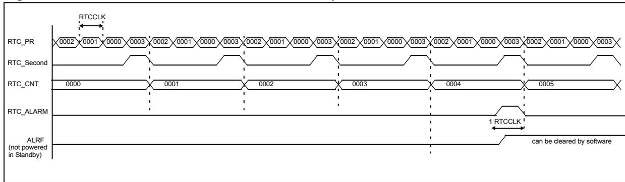
Figure 158. RTC Overflow waveform example with PR=0003
