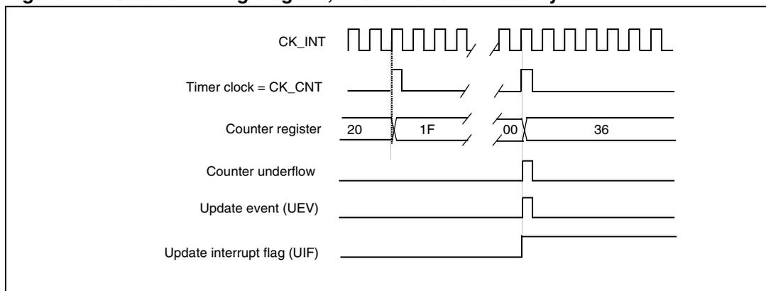
**Figure 113. Counter timing diagram, Update event when repetition counter is not used**
