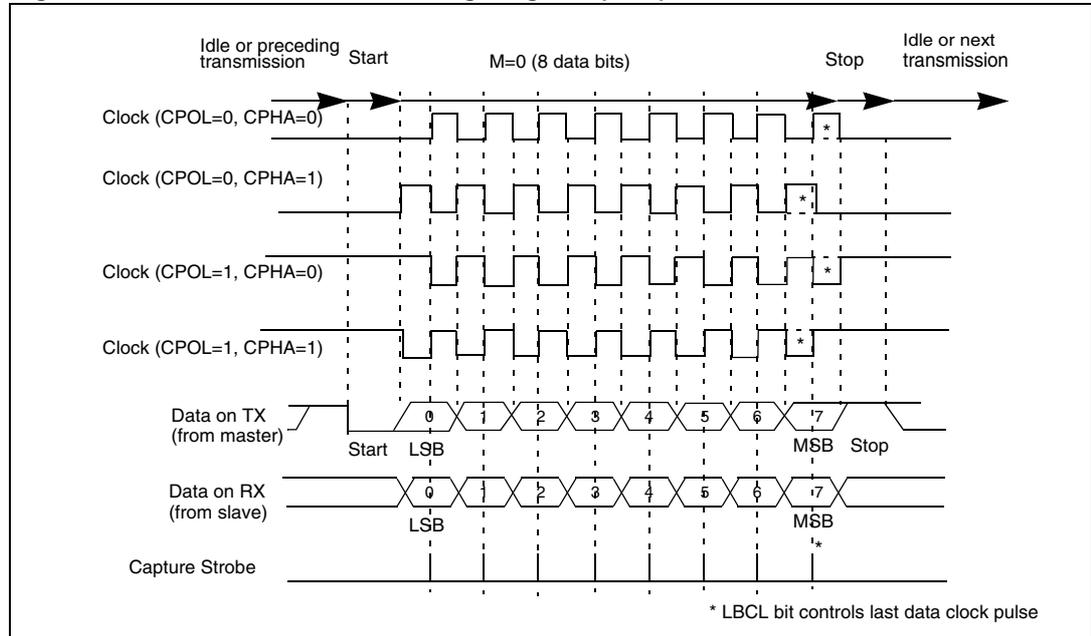
**Figure 259. USART data clock timing diagram (M=1)**
