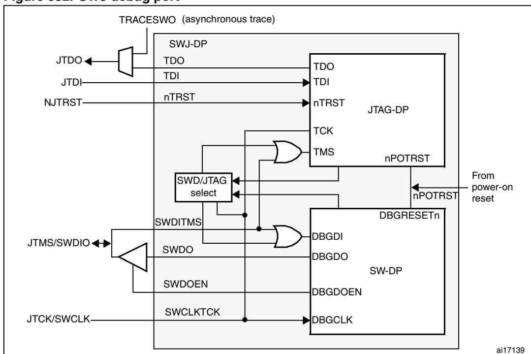
Figure 332 shows that the asynchronous TRACE output (TRACESWO) is multiplexed with TDO. This means that the asynchronous trace can only be used with SW-DP, not JTAG-DP.
