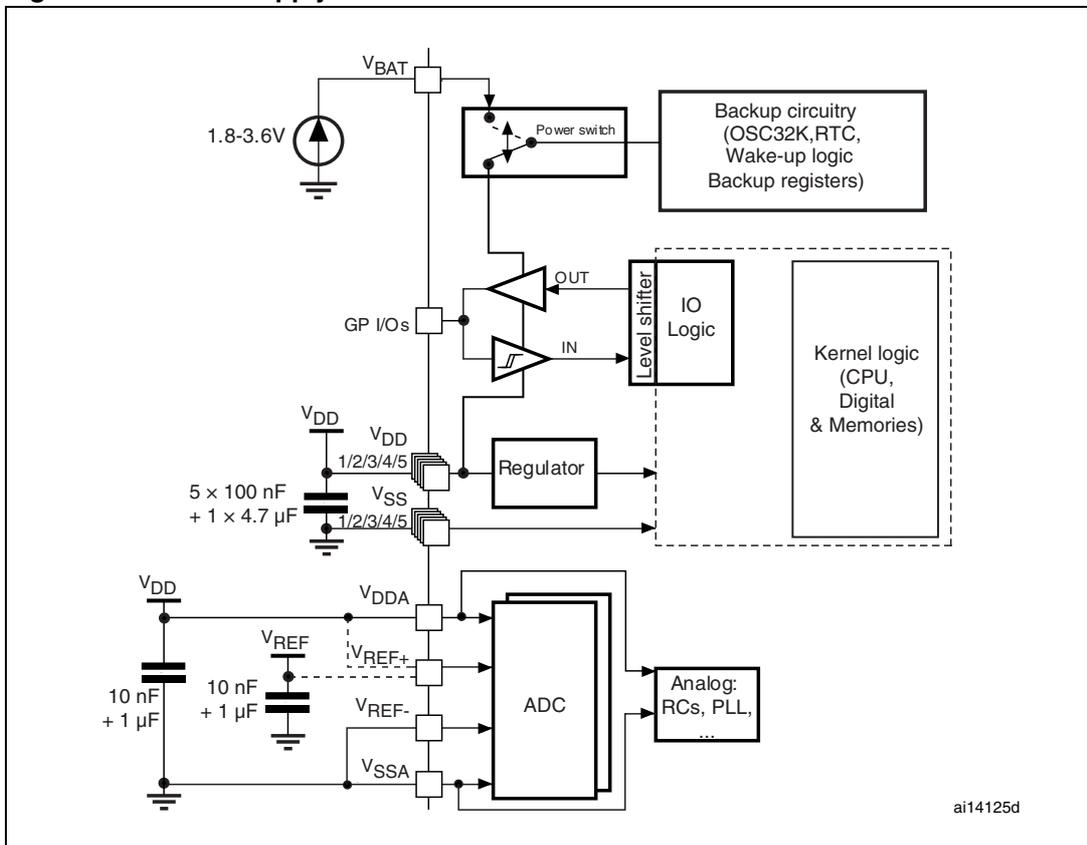
**Caution:** In [Figure 12](#), the 4.7 μF capacitor must be connected to  $V_{DD3}$ .
