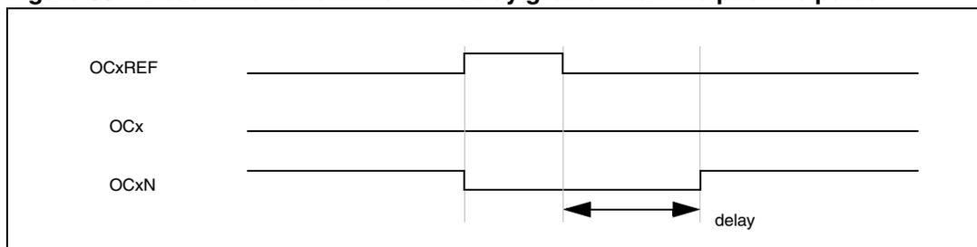
The dead-time delay is the same for each of the channels and is programmable with the DTG bits in the TIMx\_BDTR register. Refer to [Section 13.4.18: TIM1&TIM8 break and dead-time register \(TIMx\\_BDTR\) on page 317](#) for delay calculation.
