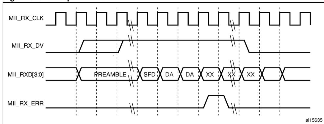
Figure 314. Reception with false carrier indication
