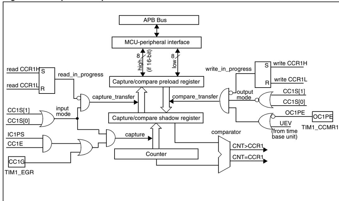
Figure 80. Output stage of capture/compare channel (channel 1 to 3)
