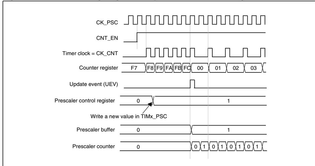
**Figure 148. Counter timing diagram with prescaler division change from 1 to 4**
