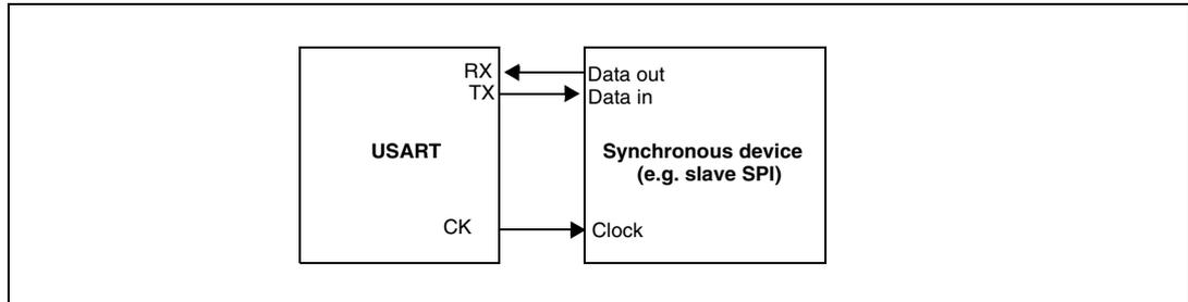
Figure 258. USART data clock timing diagram (M=0)
