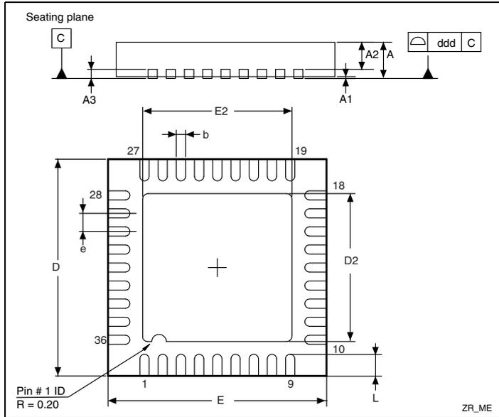
Figure 36. Recommended footprint (dimensions in mm)<sup>(1)(2)(3)</sup>
