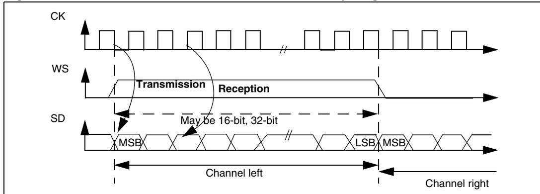
Data are latched on the falling edge of CK (for transmitter) and are read on the rising edge (for the receiver).
