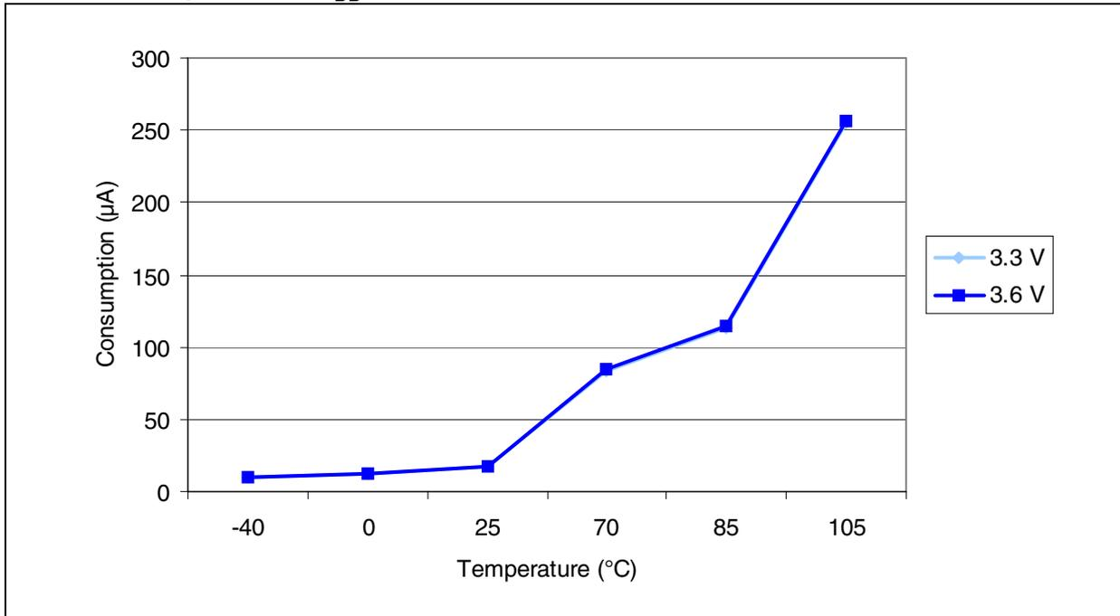
**Figure 19. Typical current consumption in Standby mode versus temperature at  $V_{DD} = 3.3\text{ V}$  and  $3.6\text{ V}$**
