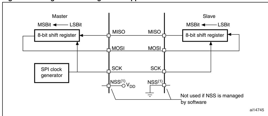
1. Here, the NSS pin is configured as an input.
