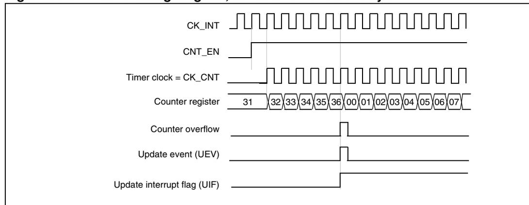
**Figure 150. Counter timing diagram, internal clock divided by 2**
