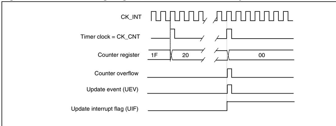
**Figure 107. Counter timing diagram, Update event when ARPE=0 (TIMx\_ARR not preloaded)**
