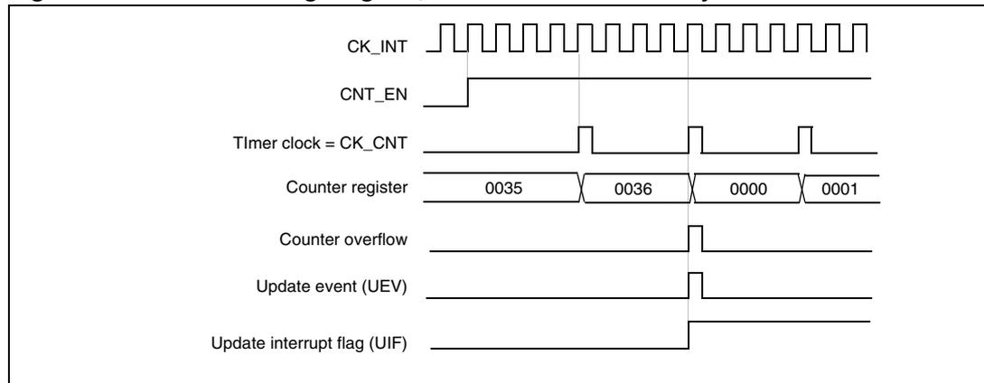
**Figure 152. Counter timing diagram, internal clock divided by N**
