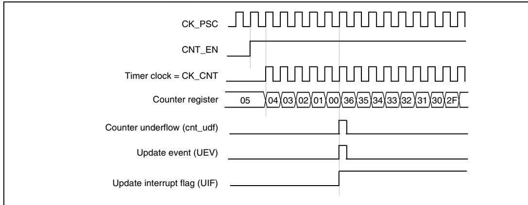
**Figure 62. Counter timing diagram, internal clock divided by 2**
