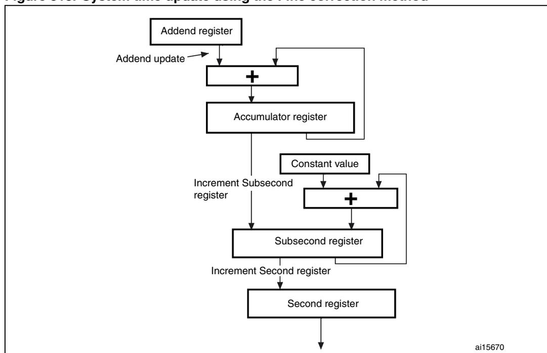
The system time update logic requires a 50 MHz clock frequency to achieve 20 ns accuracy. The frequency division is the ratio of the reference clock frequency to the required clock frequency. Hence, if the reference clock (HCLK) is, let us say, 66 MHz, the ratio is calculated as  $66 \text{ MHz}/50 \text{ MHz} = 1.32$ . Hence, the default addend value to be set in the register is  $2^{32}/1.32$ , which is equal to  $0xC1F0\ 7C1F$ .
