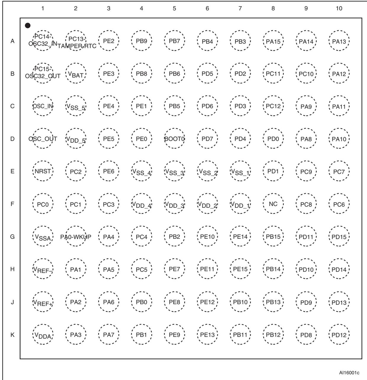
Figure 4. STM32F103xx performance line LQFP100 pinout
