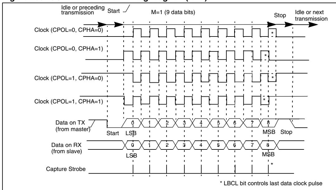
**Figure 260. RX data setup/hold time**
