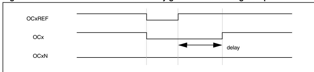
**Figure 88. Dead-time waveforms with delay greater than the positive pulse.**
