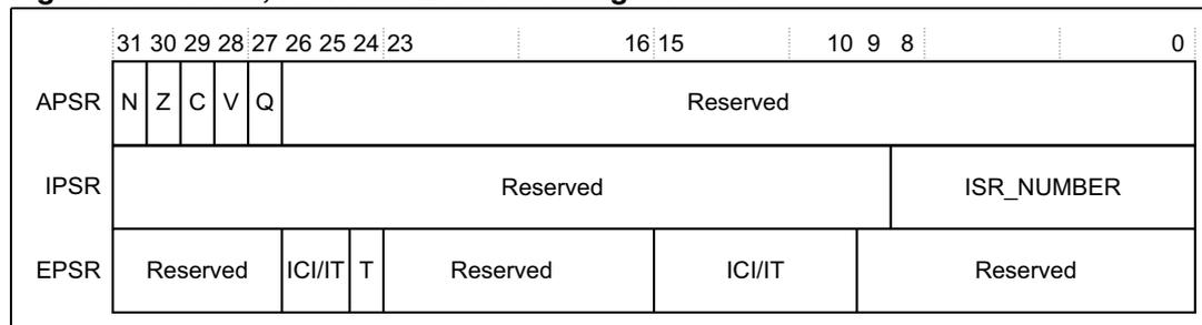
**Figure 4. PSR bit assignments**
