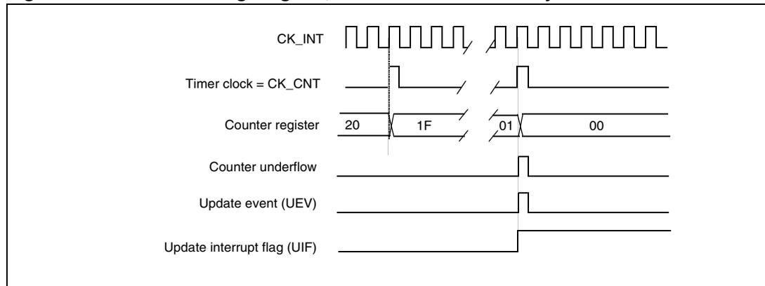
**Figure 118. Counter timing diagram, Update event with ARPE=1 (counter underflow)**
