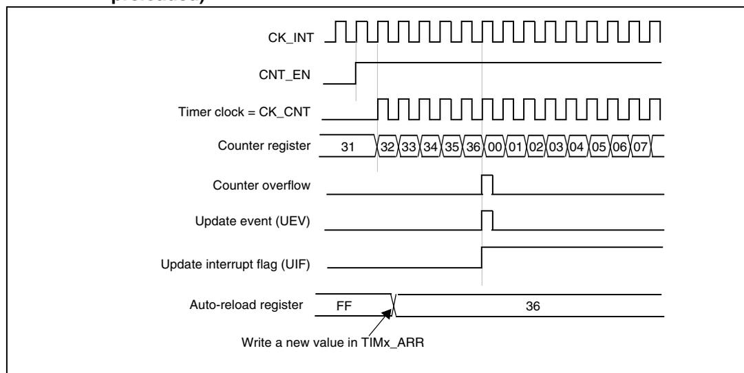
**Figure 154. Counter timing diagram, update event when ARPE=1 (TIMx\_ARR preloaded)**
