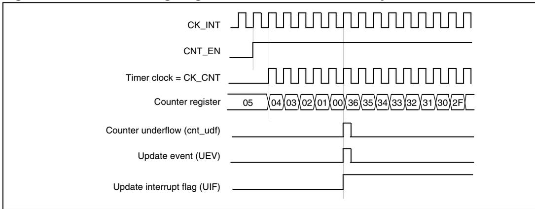
**Figure 110. Counter timing diagram, internal clock divided by 2**
