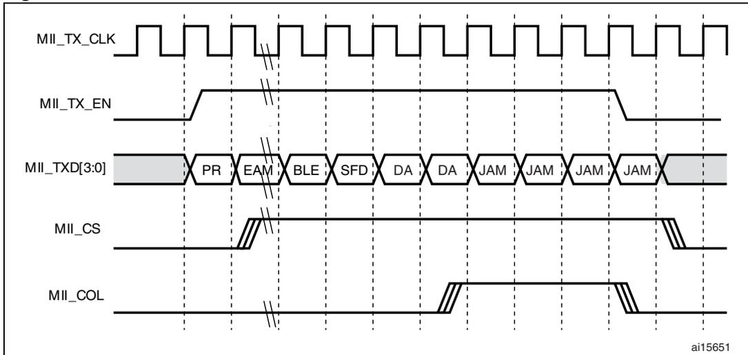
Figure 310 shows a frame transmission in MII and RMII.
