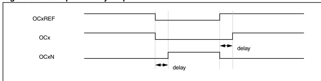
**Figure 87. Dead-time waveforms with delay greater than the negative pulse.**
