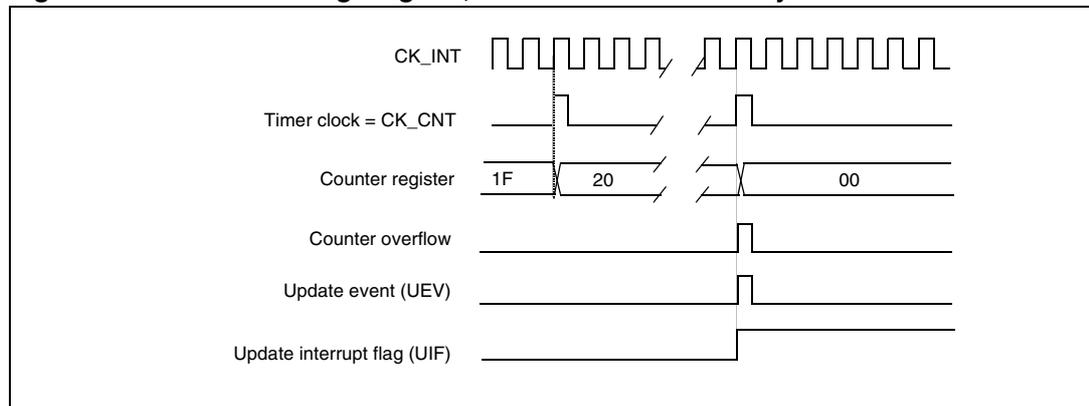
**Figure 153. Counter timing diagram, update event when ARPE = 0 (TIMx\_ARR not preloaded)**
