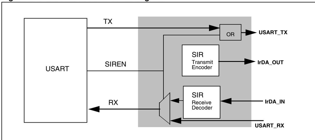
**Figure 264. IrDA data modulation (3/16) -normal mode**
