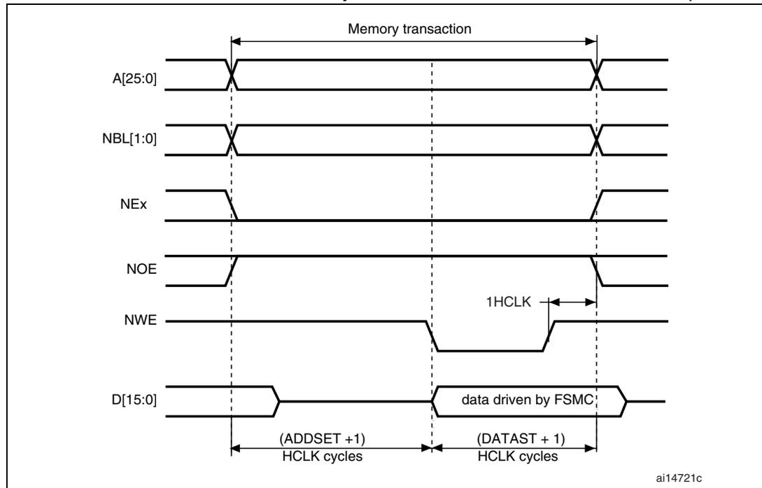
guarantee the address and data hold time after the NWE rising edge. Due to the presence of this one HCLK cycle, the DATAST value must be greater than zero (DATAST > 0).
