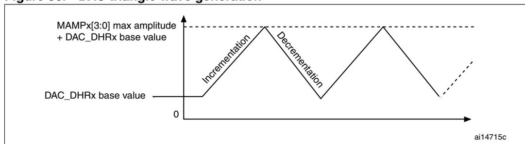
**Figure 51. DAC conversion (SW trigger enabled) with triangle wave generation**
