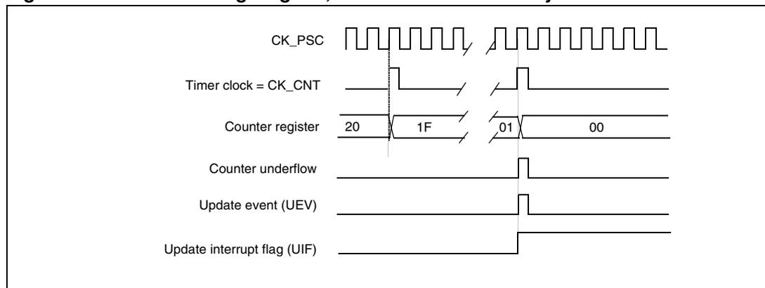
**Figure 70. Counter timing diagram, update event with ARPE=1 (counter underflow)**
