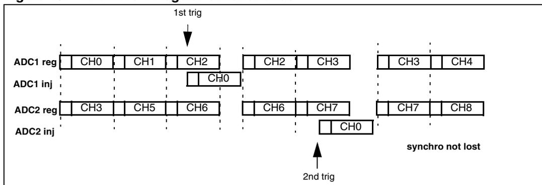
If a trigger occurs during an injected conversion that has interrupted a regular conversion, it will be ignored. [Figure 41](#) shows the behavior in this case (2nd trig is ignored).
