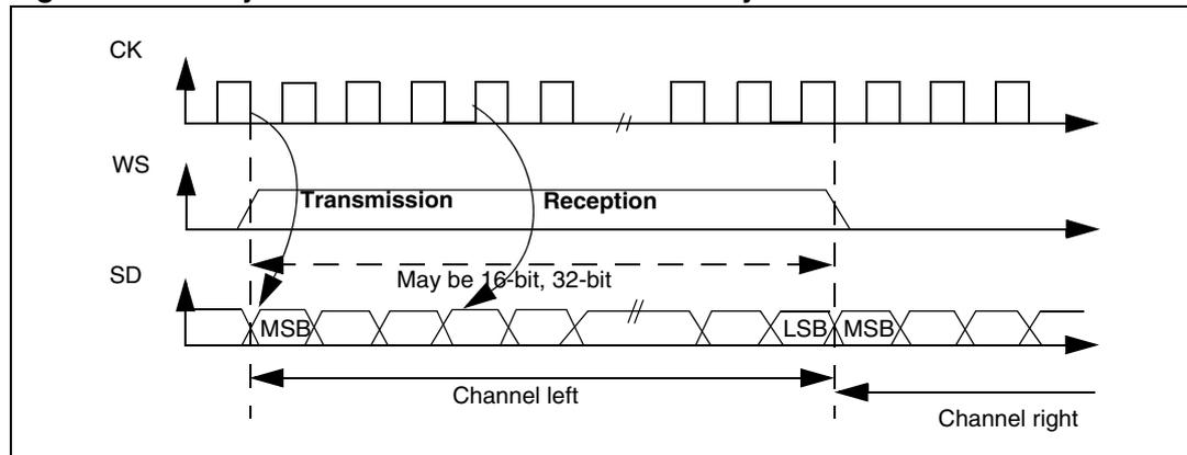
**Figure 231. LSB Justified 24-bit frame length with CPOL = 0**
