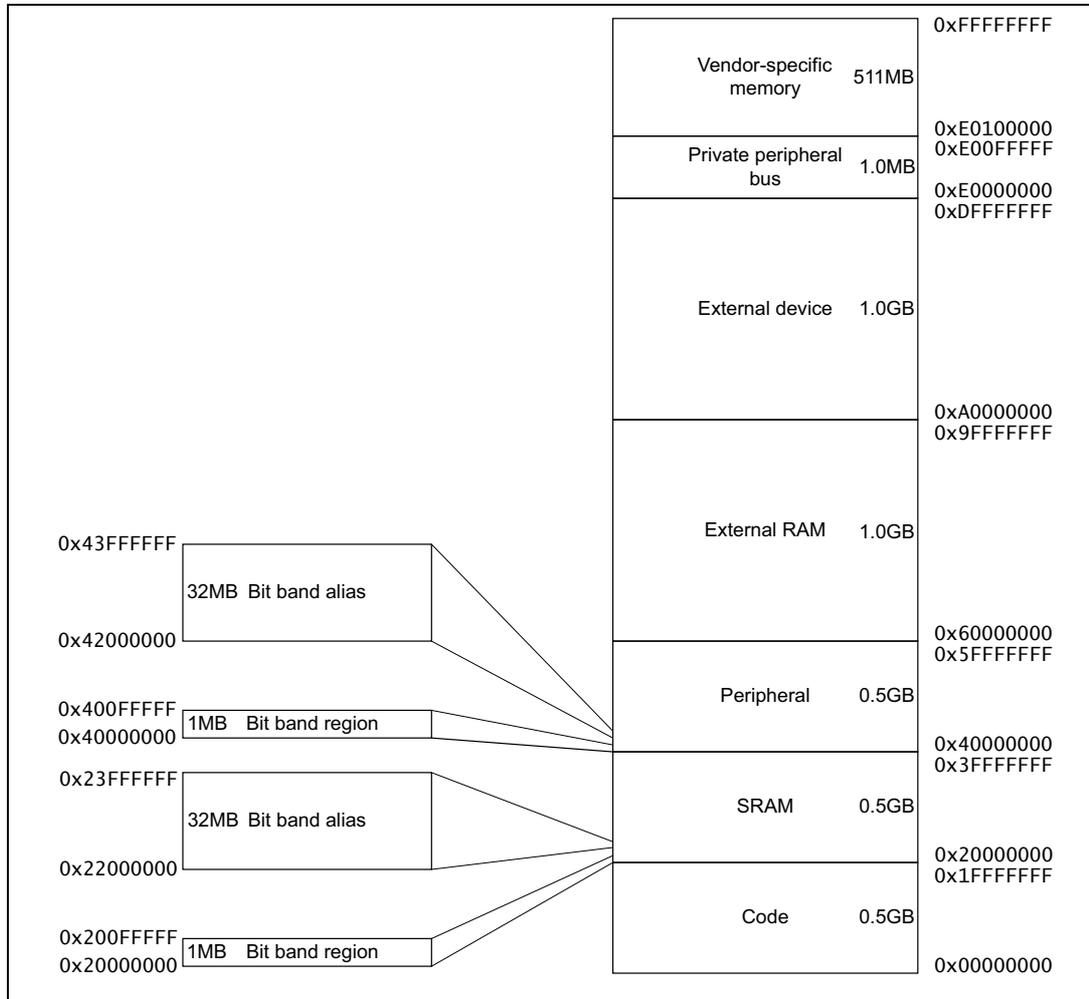
The regions for SRAM and peripherals include bit-band regions. Bit-banding provides atomic operations to bit data, see [Section 2.2.5: Bit-banding on page 27](#).
