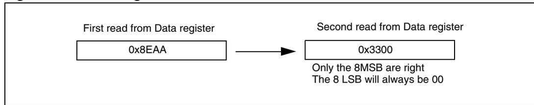
**Figure 225. I<sup>2</sup>S Phillips standard (16-bit extended to 32-bit packet frame with CPOL = 0)**
