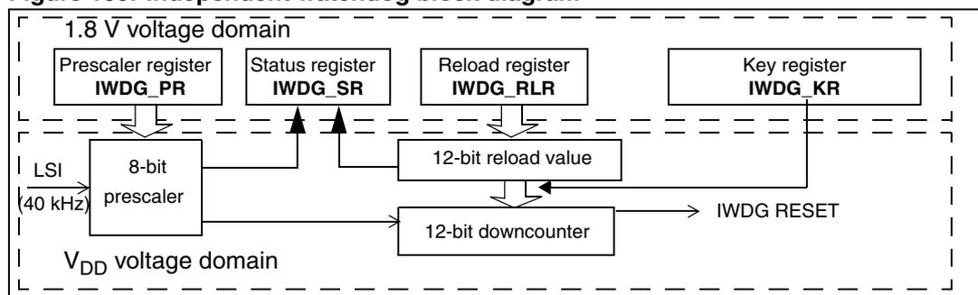
*Note:* The watchdog function is implemented in the V<sub>DD</sub> voltage domain that is still functional in Stop and Standby modes.
