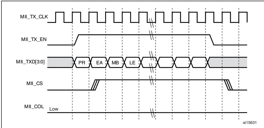
Figure 309. Transmission with collision
