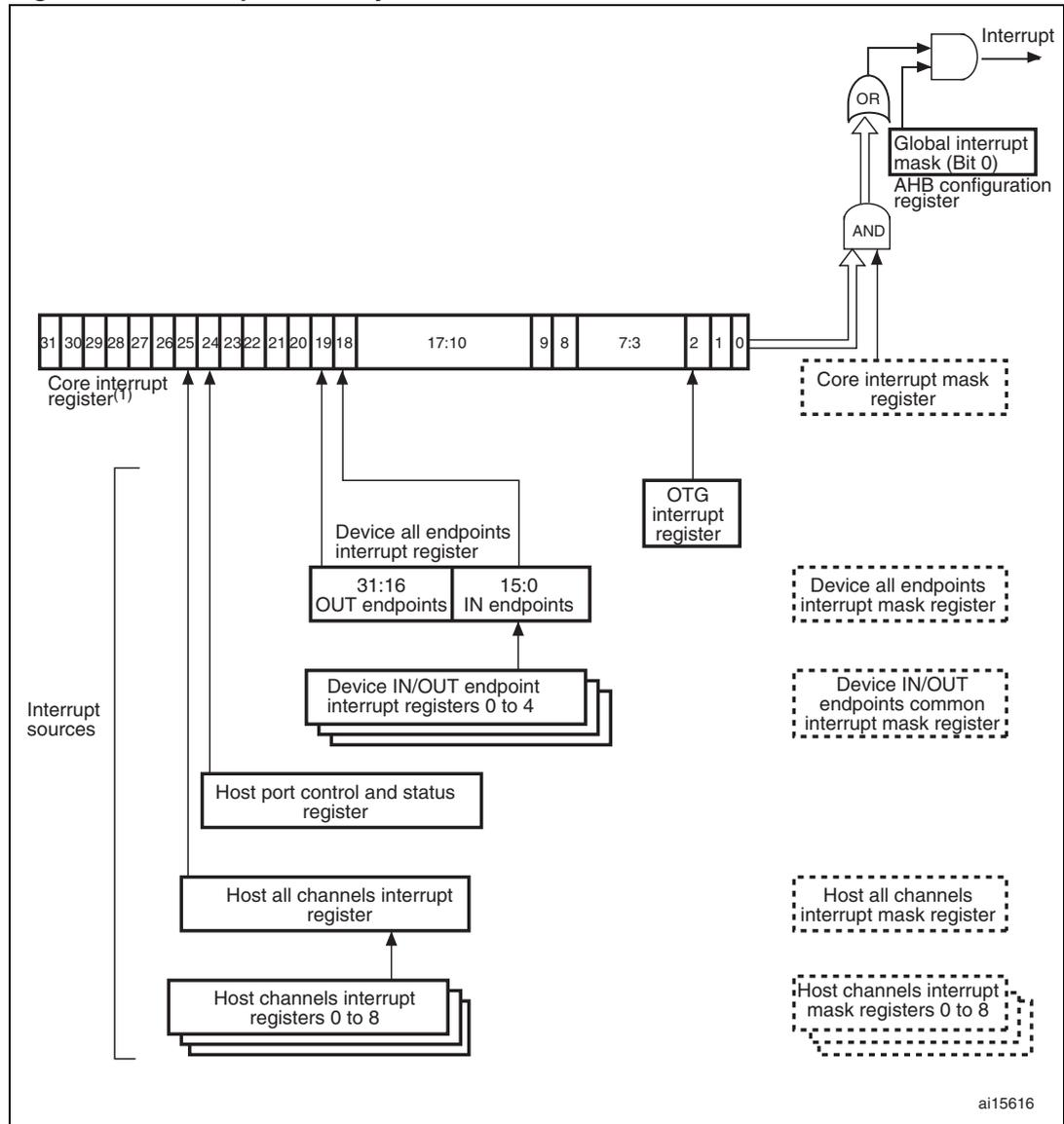
1. The core interrupt register bits are shown in *OTG\_FS core interrupt register (OTG\_FS\_GINTSTS)* on page 745.
