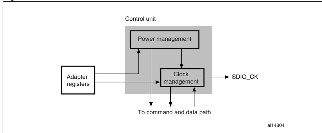
The control unit is illustrated in [Figure 185](#). It consists of a power management subunit and a clock management subunit.
