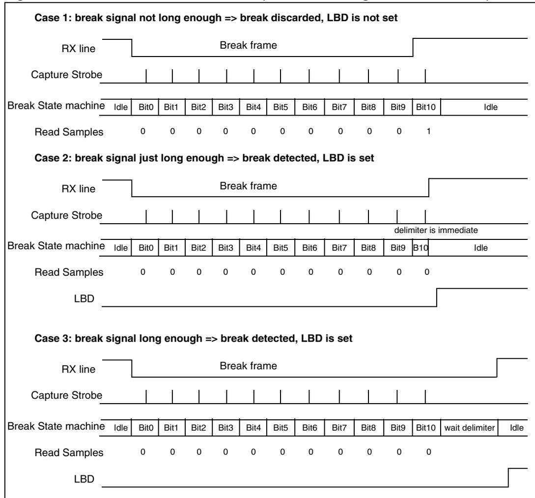
**Figure 256. Break detection in LIN mode vs. Framing error detection**
