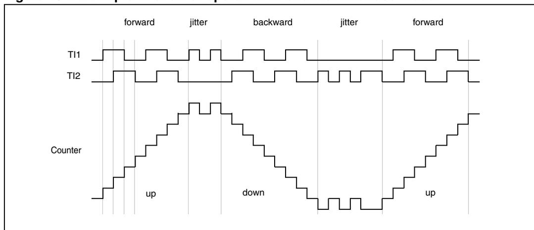
Figure 135 gives an example of counter behavior when IC1FP1 polarity is inverted (same configuration as above except CC1P=1).
