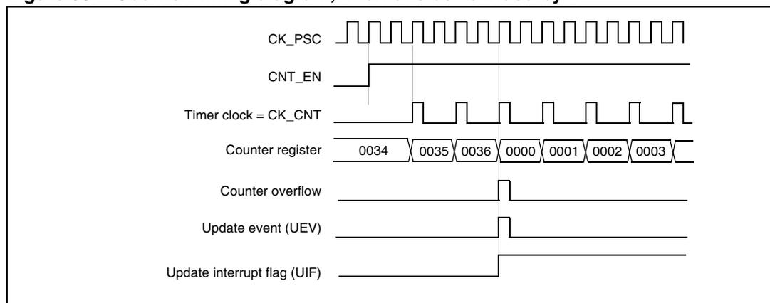
**Figure 57. Counter timing diagram, internal clock divided by 4**
