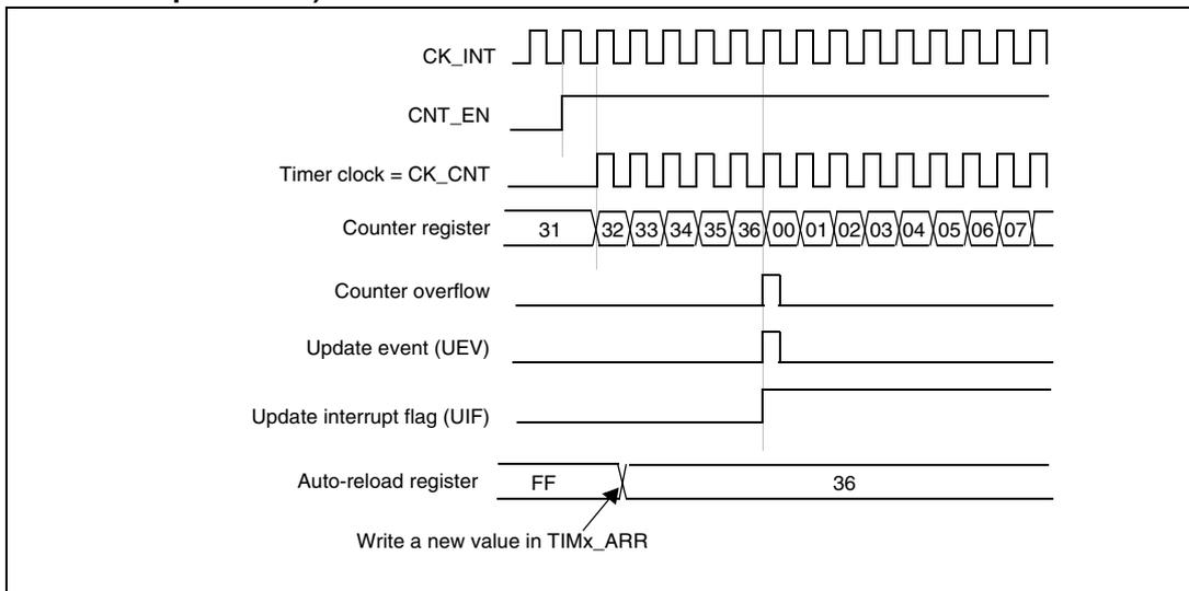
**Figure 108. Counter timing diagram, Update event when ARPE=1 (TIMx\_ARR preloaded)**
