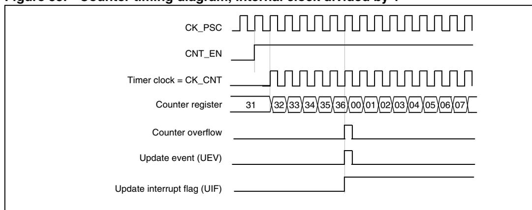
**Figure 56. Counter timing diagram, internal clock divided by 2**
