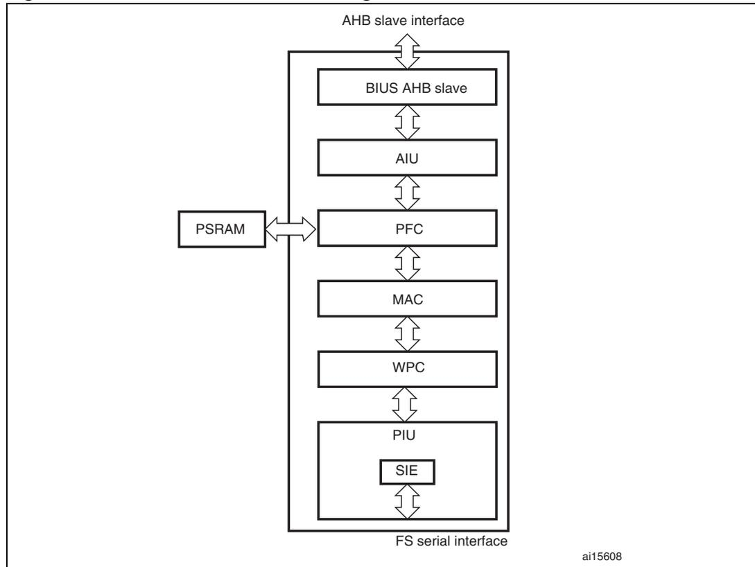
1. BIUS = bus interface unit, AIU = application interface unit, PFC = packet FIFO controller, MAC = media access controller, WPC = wakeup and power controller, PIU = PHY interface unit, SIE = serial interface engine.
