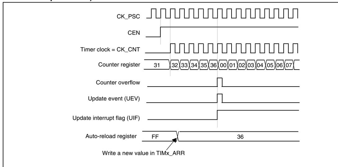
**Figure 60. Counter timing diagram, update event when ARPE=1 (TIMx\_ARR preloaded)**
