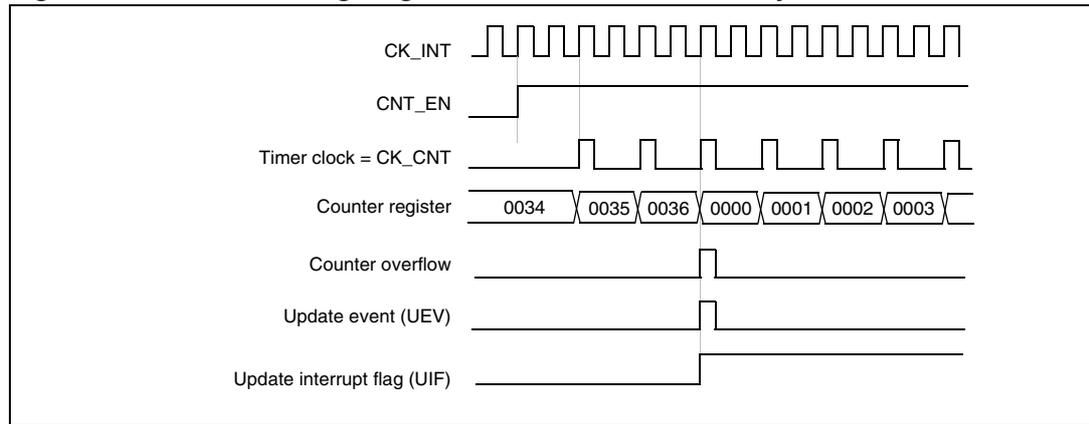
**Figure 151. Counter timing diagram, internal clock divided by 4**
