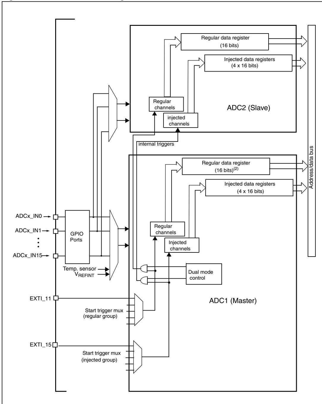
1. External triggers are present on ADC2 but are not shown for the purposes of this diagram.
