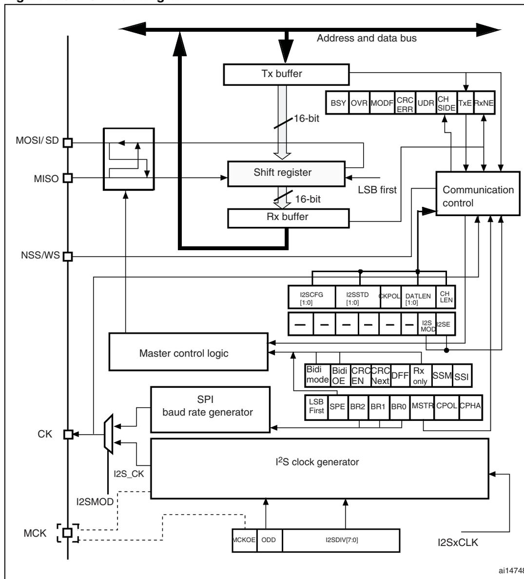
The SPI could function as an audio I<sup>2</sup>S interface when the I<sup>2</sup>S capability is enabled (by setting the I2SMOD bit in the SPI\_I2SCFGR register). This interface uses almost the same pins, flags and interrupts as the SPI.
