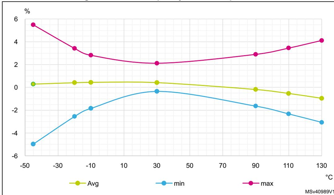
Low-speed internal (LSI) RC oscillator
