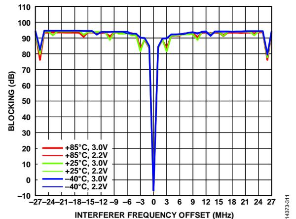
Figure 11. Receiver Wideband Blocking vs. Interferer Frequency Offset, Temperature, and  $V_{DD}$ ; Configuration 169.43125 MHz/2.4 kbps; Unmodulated Interferer; Desired Signal 3 dB Above the Sensitivity Level of PER = 5%; PER-Based Test
