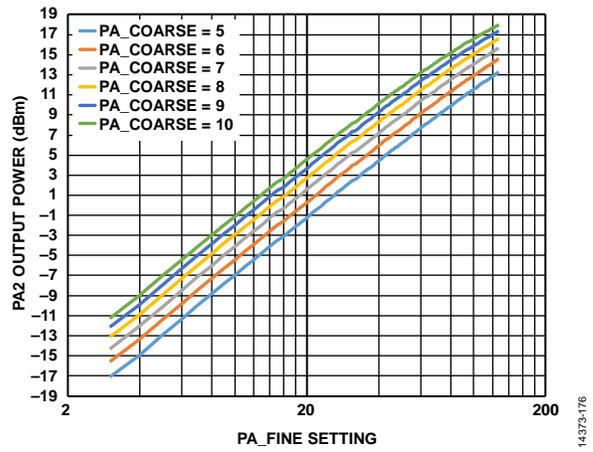
Figure 75. PA2 Output Power vs. PA\_FINE Setting and PA\_COARSE Setting with PA\_FINE on a Logarithmic Scale, PAOLDO\_VOUT\_CON = 15, RF Frequency = 915 MHz,  $V_{DD} = 3.0\text{ V}$ ,  $T_A = 25^\circ\text{C}$
