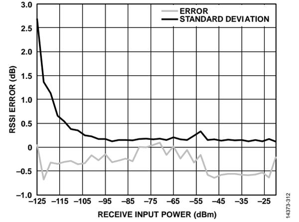
Figure 12. Packet RSSI Error vs. Rx Input Power with One-Point Calibration at  $-50\text{ dBm}$ ,  $V_{DD} = 3.0\text{ V}$ ,  $T_A = 25^\circ\text{C}$ , Configuration 169.43125 MHz/2.4 kbps (Error is Based on the Mean RSSI of 100 Packets)
