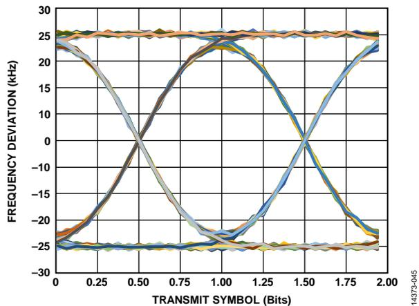
Figure 44. Transmit Eye Diagram; PA2 Output Power = 17 dBm; Configuration 460 MHz/7.2 kbps; BT = 0.5; V<sub>DD</sub> = 3.0 V; T<sub>A</sub> = 25°C
