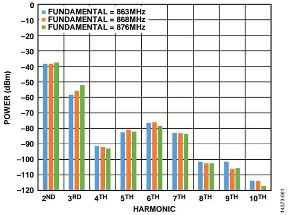
Figure 62. Conductive Harmonic Emission Level, PA2 Output Power = 17 dBm, RF Frequency = 868 MHz, V<sub>DD</sub> = 3.0 V, T<sub>A</sub> = 25°C
