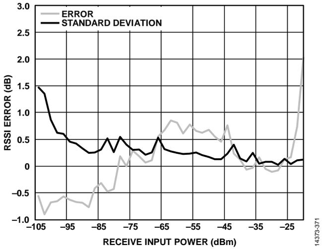
Figure 71. Packet RSSI Error vs. Rx Input Power with One-Point Calibration at -70 dBm; Configuration 915 MHz/150 kbps;  $V_{DD} = 3.0\text{ V}$ ;  $T_A = 25^\circ\text{C}$  (Error is Based on the Mean RSSI of 100 Packets)
