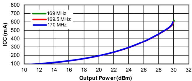
**Figure 6. Icc vs Pout, CW**
