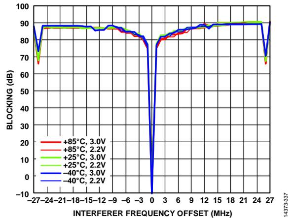
Figure 37. Receiver Wideband Blocking vs. Interferer Frequency Offset, Temperature, and  $V_{DD}$ ; Configuration 460 MHz/7.2 kbps; Unmodulated Interferer; Desired Signal 3 dB Above the Sensitivity Level of PER = 5%; PER-Based Test
