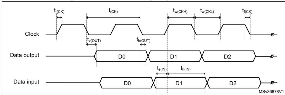
Figure 36. Quad SPI timing diagram - DDR mode
