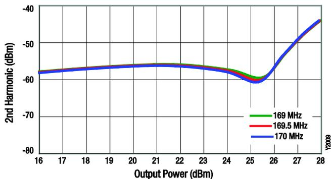
Figure 9. 2<sup>nd</sup> Harmonic vs Pout
