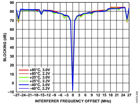
Figure 25. Receiver Wideband Blocking vs. Interferer Frequency Offset, Temperature, and  $V_{DD}$ ; Configuration 433 MHz/50 kbps; Unmodulated Interferer; Desired Signal 3 dB Above the Sensitivity Level of PER = 5%; PER-Based Test
