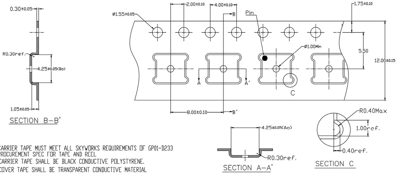
1. CARRIER TAPE MUST MEET ALL SKYWORKS REQUIREMENTS OF GP01-D233 PROCUREMENT SPEC FOR TAPE AND REEL
