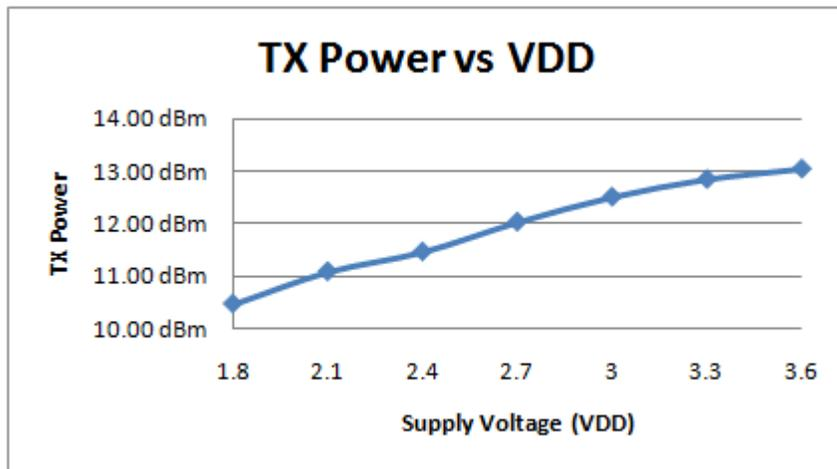
Figure 14. +13 dBm TX Power vs. Supply Voltage (VDD)
