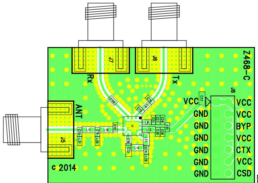
**Figure 14. SKY66100-11 Evaluation Board Assembly Drawing
