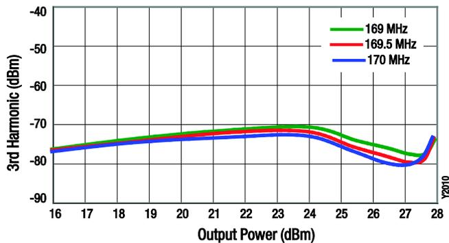
Figure 10. 3<sup>rd</sup> Harmonic vs Pout
