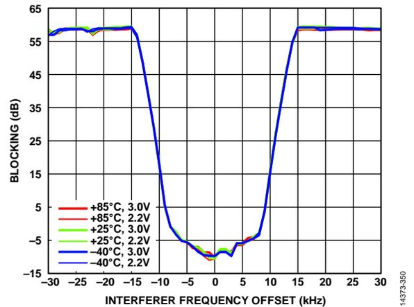
Figure 50. Receiver Close-In Blocking vs. Interferer Frequency Offset, Temperature, and  $V_{DD}$ ; Configuration 868 MHz/4.8 kbps, Unmodulated Interferer; Desired Signal 3 dB Above the Sensitivity Level of PER = 5% PER-Based Test
