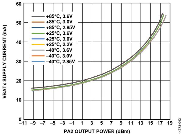
Figure 41. VBATx Supply Current vs. PA2 Output Power, Temperature, and V<sub>DD</sub> with PA\_COARSE = 10, PAOLDO\_VOUT\_CON = 15, RF Frequency = 460 MHz
