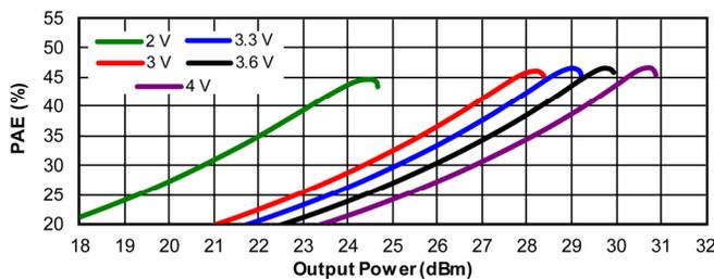
**Figure 7. PAE vs Pout and Vcc, CW**
