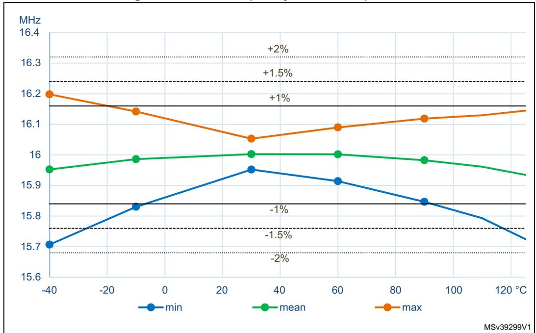
Multi-speed internal (MSI) RC oscillator
