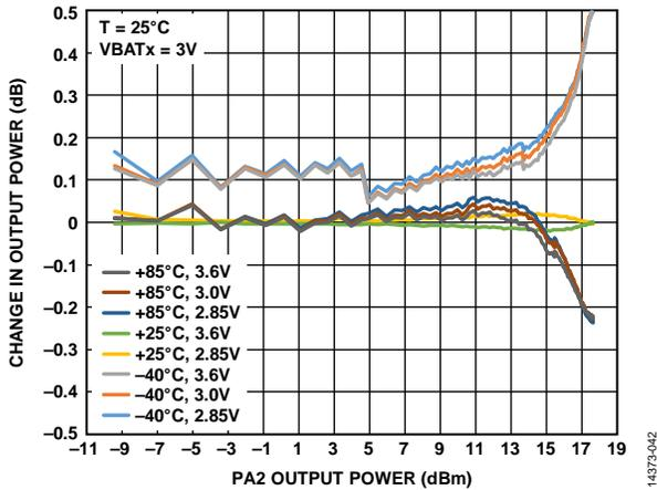
Figure 40. Change in PA2 Output Power vs. Temperature, and V<sub>DD</sub> with PA\_COARSE = 10, PAOLDO\_VOUT\_CON=15, RF Frequency = 460 MHz; Variation Above 15 dBm Can Be Improved by Matching the PA for Higher Output Power
