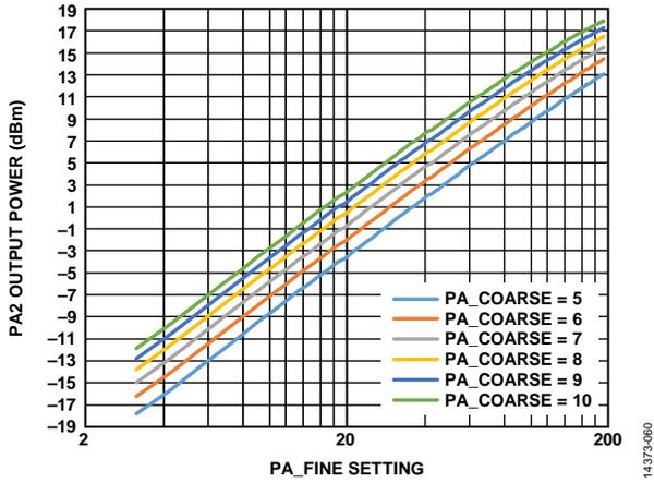
Figure 61. PA2 Output Power vs. PA\_FINE Setting and PA\_COARSE Setting with PA\_FINE on a Logarithmic Scale, PAOLDO\_VOUT\_CON = 15, RF Frequency = 868 MHz, V<sub>DD</sub> = 3.0 V, T<sub>A</sub> = 25°C
