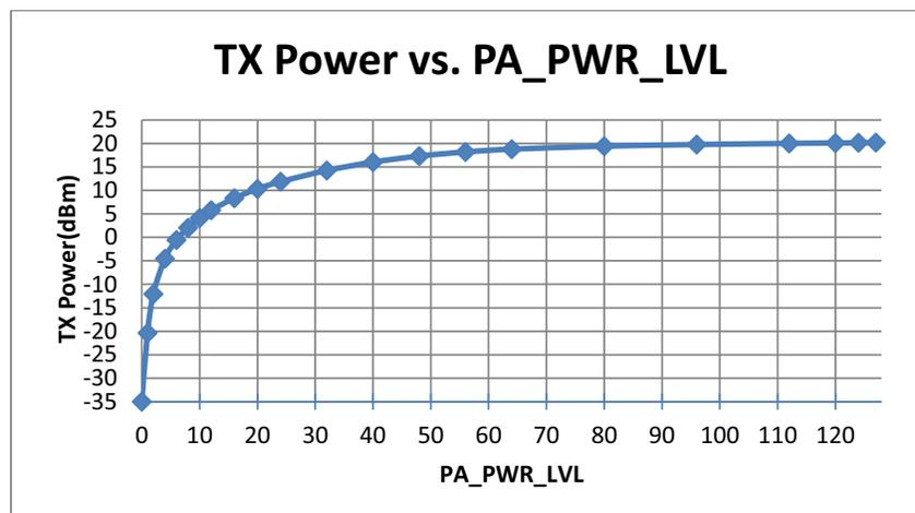
Figure 10. +20 dBm TX Power vs. PA\_PWR\_LVL
