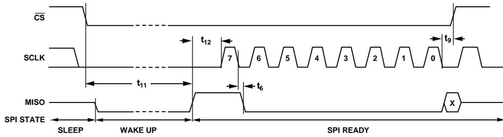
Figure 3. PHY\_SLEEP to SPI Ready State Timing
