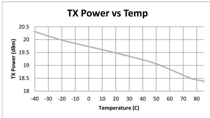
Figure 12. +20 dBm TX Power vs. Temp
