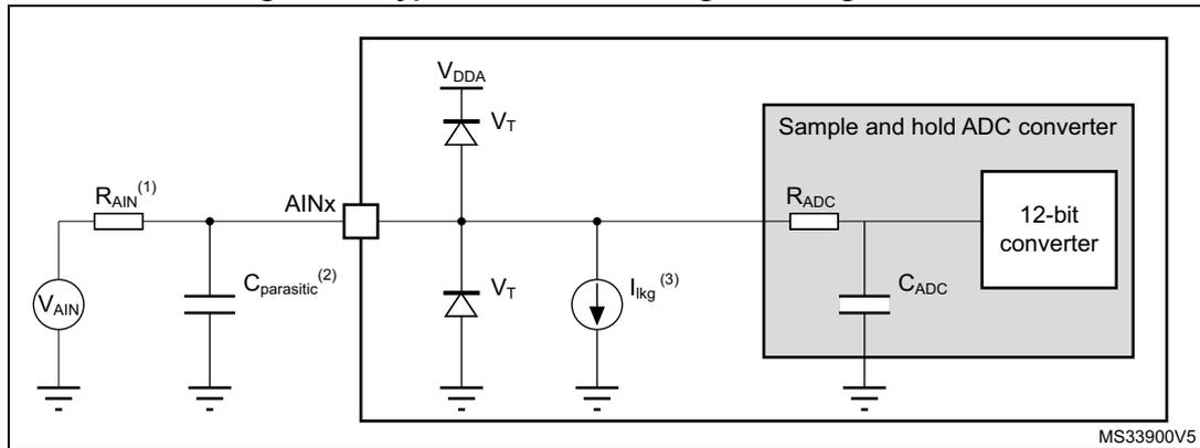
1. Refer to [Table 67: ADC characteristics](#) for the values of  $R_{AIN}$  and  $C_{ADC}$ .
