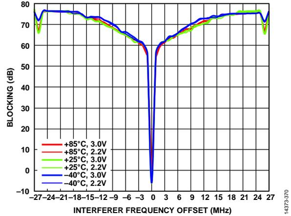
Figure 70. Receiver Wideband Blocking vs. Interferer Frequency Offset, Temperature, and  $V_{DD}$ ; Configuration 915 MHz/150 kbps; Unmodulated Interferer; Desired Signal 3 dB Above the Sensitivity Level of PER = 5%; PER-Based Test
