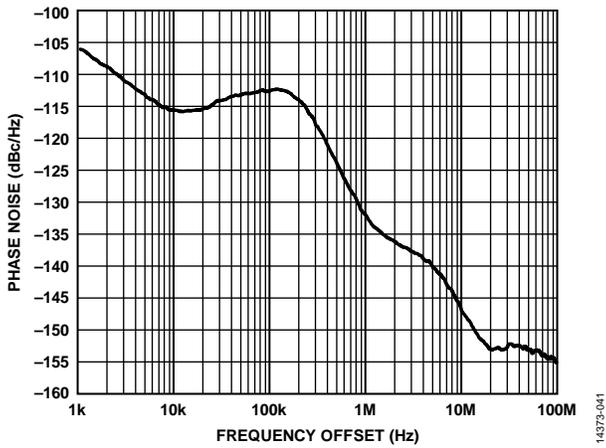
Figure 39. Phase Noise vs. Frequency Offset, RF Frequency = 460 MHz, PA2 Output Power = 17 dBm, V<sub>DD</sub> = 3.0 V, T<sub>A</sub> = 25°C
