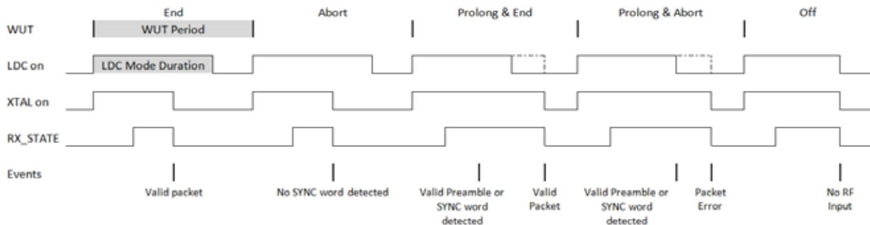
**Figure 19. Low Duty Cycle Mode for RX**
