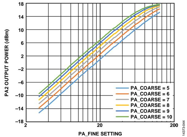
Figure 42. PA2 Output Power vs. PA\_FINE Setting and PA\_COARSE Setting with PA\_FINE on a Logarithmic Scale, PAOLDO\_VOUT\_CON=15, RF Frequency = 460 MHz, V<sub>DD</sub> = 3.0 V, T<sub>A</sub> = 25°C
