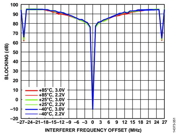
Figure 51. Receiver Wideband Blocking vs. Interferer Frequency Offset, Temperature, and  $V_{DD}$ ; Configuration 868 MHz/4.8 kbps, Unmodulated Interferer; Desired Signal 3 dB Above the Sensitivity Level of PER = 5% PER-Based Test
