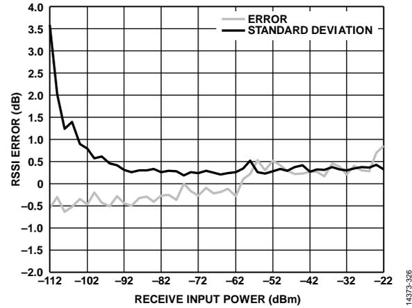
Figure 26. Packet RSSI Error vs. RX Input Power with One-Point Calibration at  $-77\text{ dBm}$ ; Configuration 433 MHz/50 kbps;  $V_{DD} = 3.0\text{ V}$ ;  $T_A = 25^\circ\text{C}$  (Error is Based on the Mean RSSI of 100 Packets)
