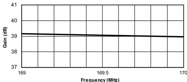
**Figure 5. Small Signal Gain vs Frequency, CW**
