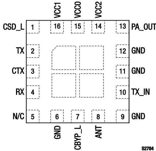
Figure 2. SKY66100-11 Pinout - 16-Pin MCM (Top View)
