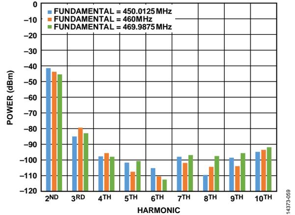
Figure 43. Conductive Harmonic Emission Level, PA2 Output Power = 17 dBm, RF Frequency = 460 MHz, V<sub>DD</sub> = 3.0 V, T<sub>A</sub> = 25°C
