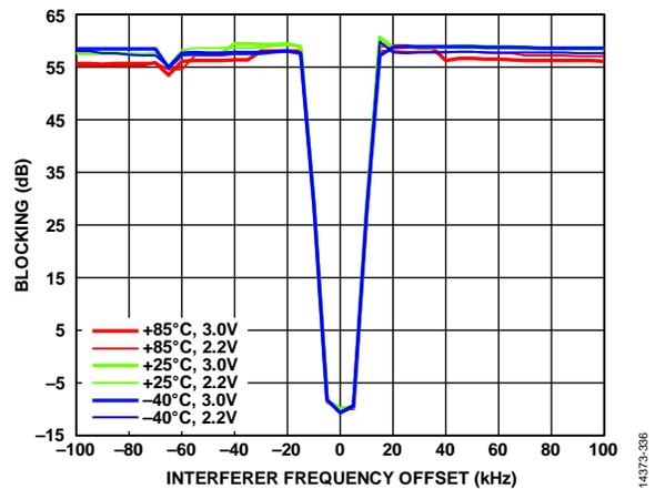
Figure 36. Receiver Close-In Blocking vs. Interferer Frequency Offset and Temperature and  $V_{DD}$ ; Configuration 460 MHz/7.2 kbps; Unmodulated Interferer; Desired Signal 3 dB Above the Sensitivity Level of PER = 5%; PER-Based Test
