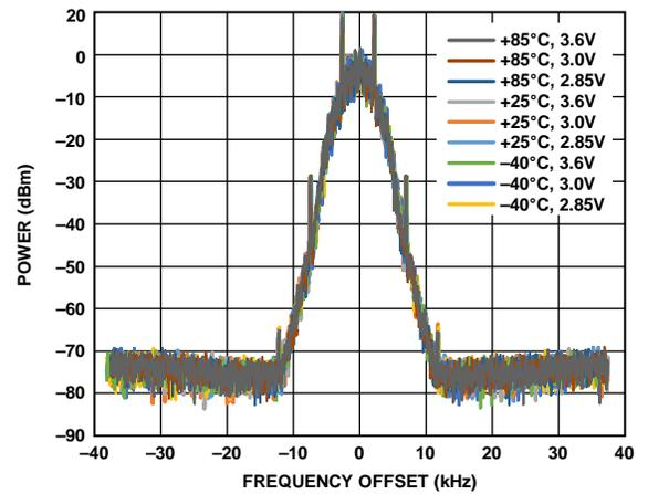
Figure 64. Transmit Spectrum vs. Temperature, and V<sub>DD</sub> with PA2 Output Power = 17 dBm, Configuration 868 MHz/4.8 kbps, V<sub>DD</sub> = 3.0 V; T<sub>A</sub> = 25°C
