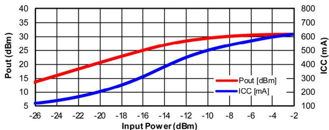
**Figure 3. Pout and Icc vs Pin, CW**
