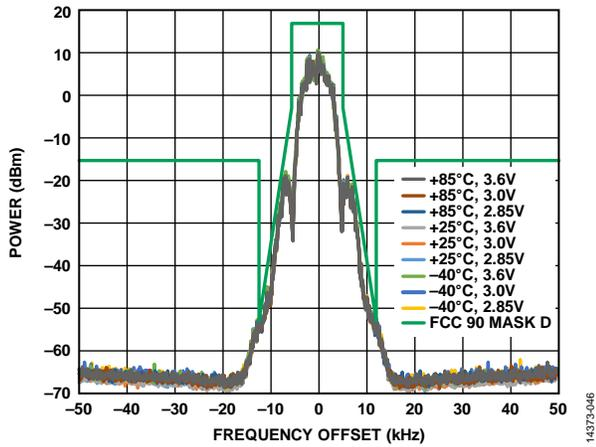
Figure 45. Transmit Spectrum, PA2 Output Power = 17 dBm, Configuration 460 MHz/7.2 kbps, BT = 0.5,  $V_{DD} = 3.0\text{ V}$ ,  $T_A = 25^\circ\text{C}$ ; Margin to the Mask Can Be Improved by Reducing the BT or By Reducing the Data Rate
