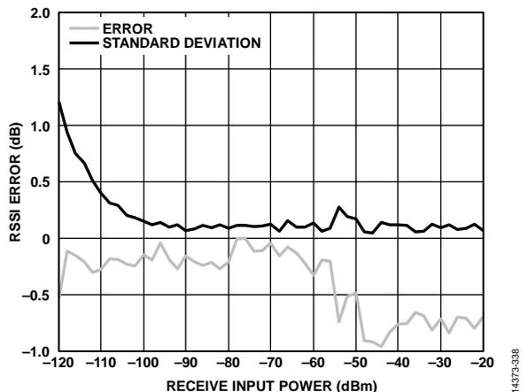
Figure 38. Packet RSSI Error vs. RF Input Power with One-Point Calibration at  $-77\text{ dBm}$ ; Configuration 460 MHz/7.2 kbps, 7.2 kbps;  $V_{DD} = 3.0\text{ V}$ ;  $T_A = 25^\circ\text{C}$  (Error is Based on the Mean RSSI of 100 Packets)
