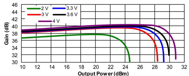
**Figure 8. Gain vs Pout and Vcc, CW**
