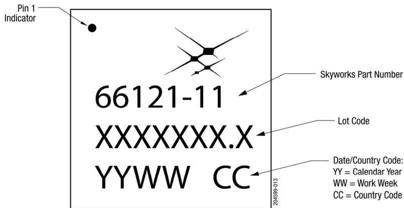
**Figure 13. Typical Part Marking**
