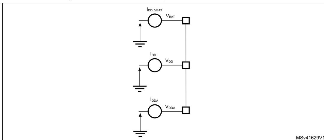
The  $I_{DD\_ALL}$  parameters given in [Table 27](#) to [Table 39](#) represent the total MCU consumption including the current supplying  $V_{DD}$ ,  $V_{DDA}$  and  $V_{BAT}$ .
