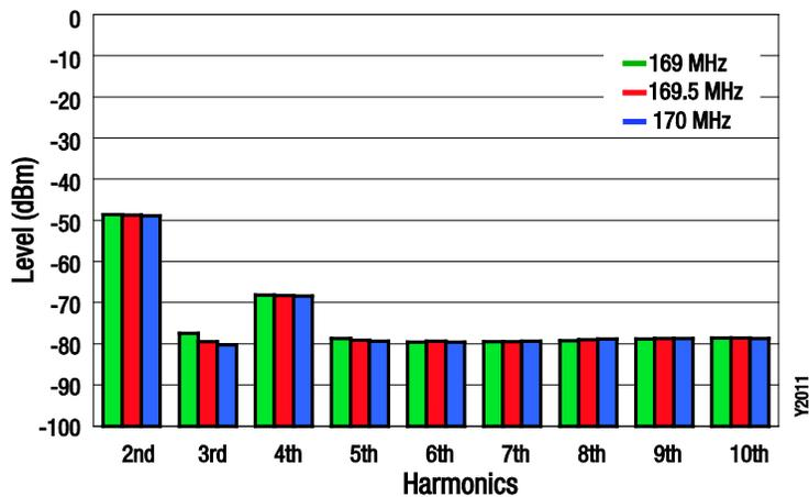
Figure 11. Harmonics at POUT = +27 dBm
