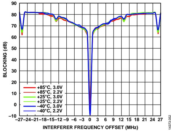
Figure 52. Receiver Wideband Blocking vs. Interferer Frequency Offset, Temperature,  $V_{DD}$ ; Configuration 868 MHz/100 kbps; Unmodulated Interferer; Desired Signal 3 dB Above the Sensitivity Level of PER = 5%; PER-Based Test
