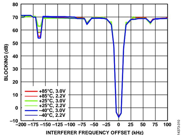
Figure 10. Receiver Close-In Blocking vs. Interferer Frequency Offset, Temperature, and  $V_{DD}$ ; Configuration 169.43125 MHz/2.4 kbps; Unmodulated Interferer; Desired Signal 3 dB Above the Sensitivity Level of PER = 5%; PER-Based Test
