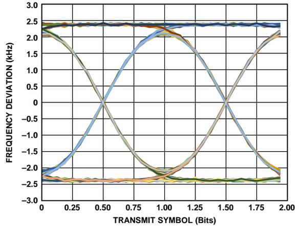
Figure 63. Transmit Eye Diagram, PA2 Output Power = 17 dBm, Configuration 868 MHz/4.8 kbps; V<sub>DD</sub> = 3.0 V; T<sub>A</sub> = 25°C
